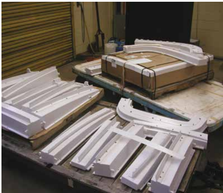
Left: A future leading-edge tool for a C-5 cargo plane. Right: Examples of 16 aircraft additive manufacturing tools that are up to 9-feet long when assembled.
