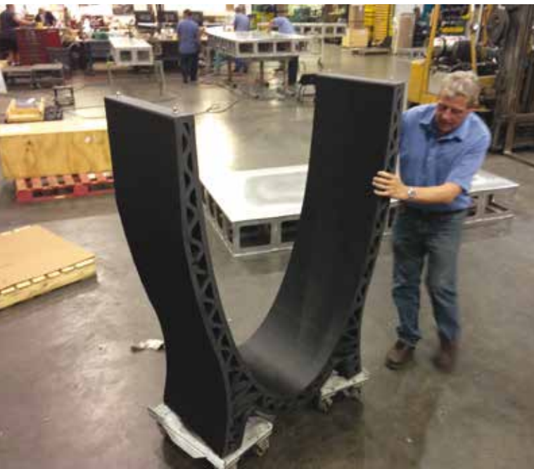
Left: A future leading-edge tool for a C-5 cargo plane. Right: Examples of 16 aircraft additive manufacturing tools that are up to 9-feet long when assembled.
