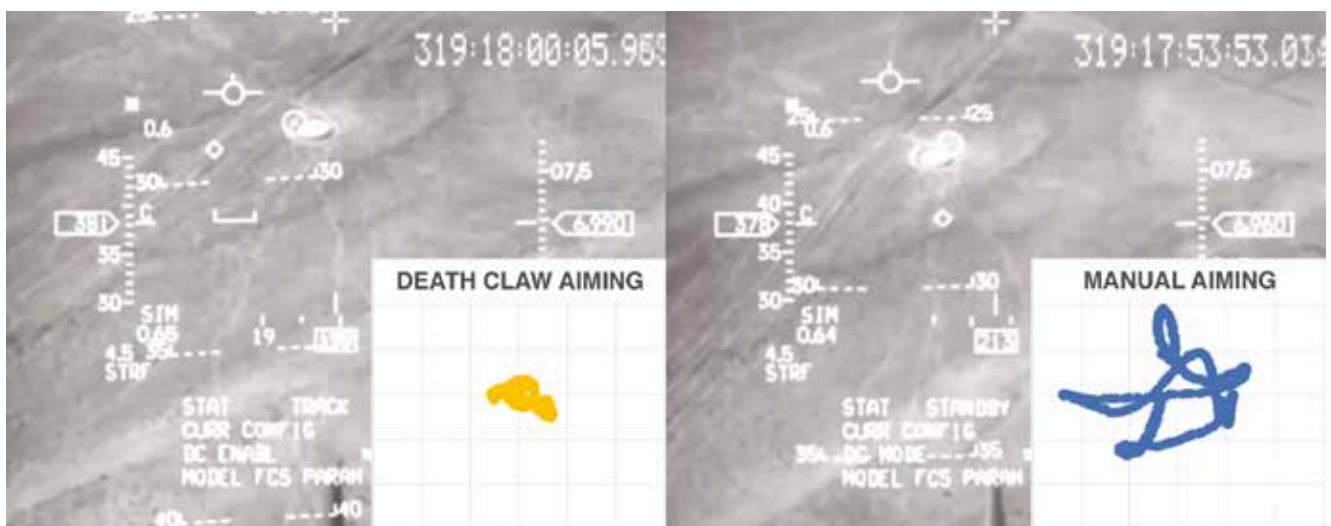
VISTA Heads Up Display images overlaid with data showing a precise comparison between DEATH CLAW and manual pilot tracking.
