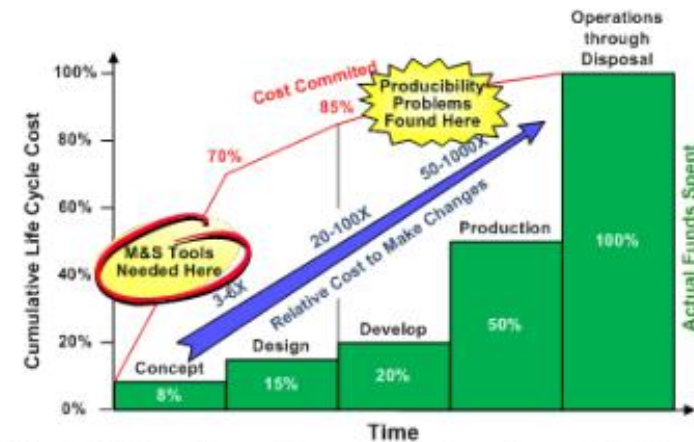
Figure 1: Life Cycle Cost Commitment as a Function of the System Life Cycle
