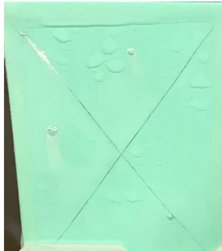
Figure 3. Pictures of a 2" × 3" test panel with LIS pre-treatment after 500h salt spray exposure.
