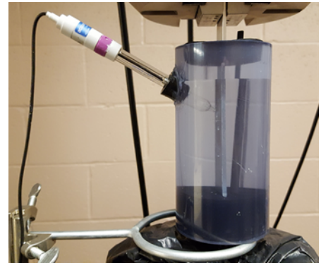
Figure 3 in situ EIS test cell
