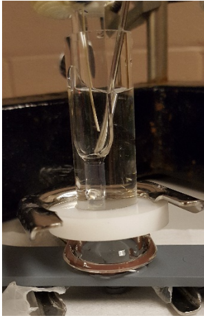
Figure 2 small paint test cell
