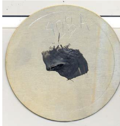
Figure 11: Conversion coating dry line
