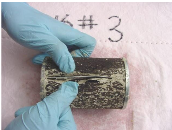
Figure 5: Paint chip contaminated fuel filter removed from a B-52 aircraft (Tinker-AFB)
