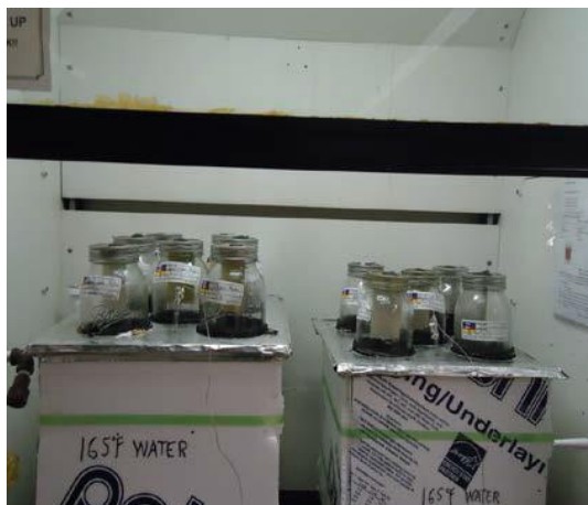
Figure 16: Test apparatus, only solution heated.
