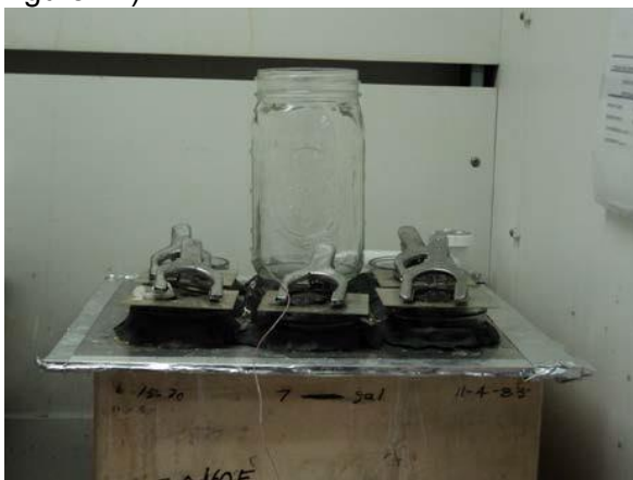
Figure 12: Test apparatus with the tops of the jars subjected to ambient conditions
