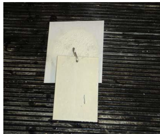
Figure 13: Vertical panel intact and the horizontal panel blistering
