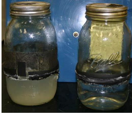
Example of the leaching of a coating
