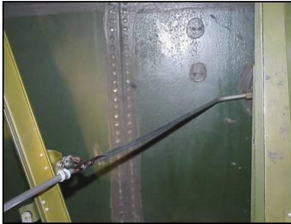
Figure 3: Fuel tank topcoat blistering in a P-3 aircraft (FRC-SE)
