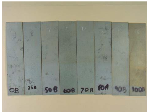
Figure 9: Panels showing depletion of chromate conversion coating with increasing water concentration left to right is decreasing water concentration.
