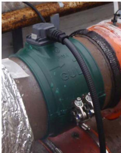
Figure 7: New design PIMS collar does not require any epoxy resins to install and has a more robust subsurface connection point.
