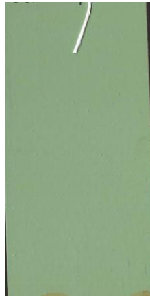
Figure 2: Polyamide epoxy primer on abraded white steel with and without vapor phase corrosion inhibitor added after 500 hours in salt fog chamber
