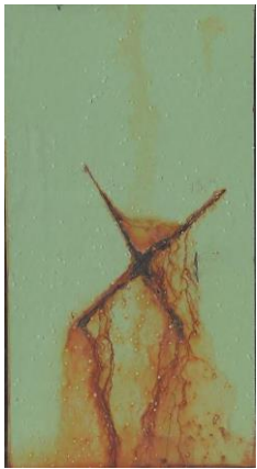
Figure 2: Polyamide epoxy primer on abraded white steel with and without vapor phase corrosion inhibitor added after 500 hours in salt fog chamber
