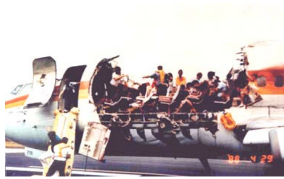
FIGURE 1. Aloha flight 243 after corrosion and metal fatigue compromised the integrity of the cabin
